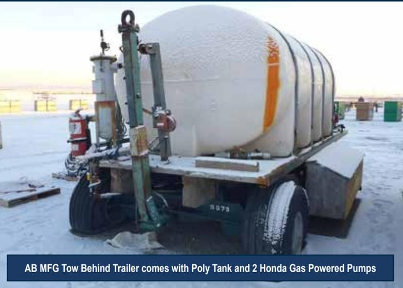
AB MFG Tow Behind Trailer comes with Poly Tank and 2 Honda Gas Powered Pumps
