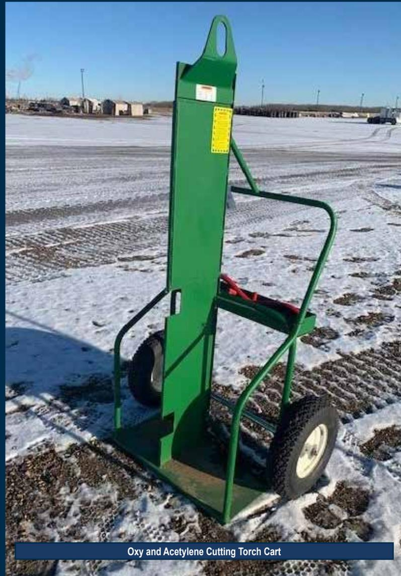
Oxy and Acetylene Cutting Torch Cart
